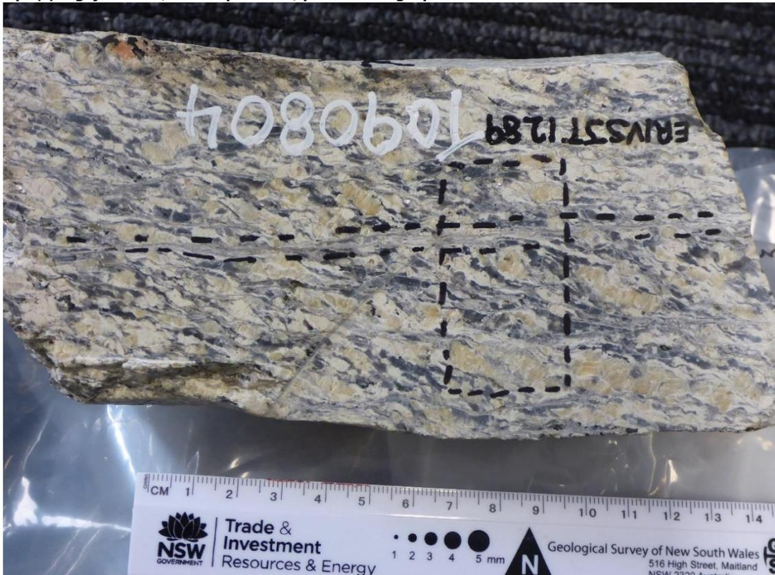
Figure 1 View onto cut surface oriented perpendicular to foliation and parallel to lineation. The penetrative S-fabric (oriented bottom-right to top-left) wraps around pale-greenish-yellow feldspar porphyroclasts. C-planes (oriented left-to-right and highlighted by parallel dashed lines) are defined by secondary sericite.
