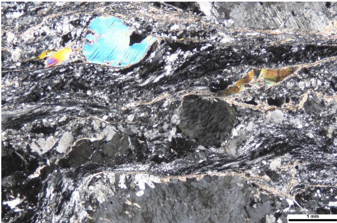
Figure 4 Photomicrograph in cross-polarised light showing a K-feldspar porphyroblast (bottom-centre) with albite replacements along the upper left margin, which is wrapped by a fine-grained aggregate of dynamically recrystallised quartz defining a C-plane shear band (oriented left-to-right). There is also muscovite fish (upper-left and right-of-centre) localised along the foliation with distinct kinks locally (e.g. right-of-centre).
